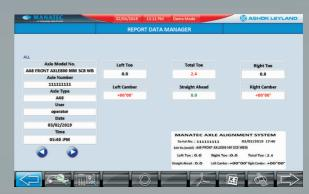
Data manager software for storing Axle alignment results with reference to Axle ID / Date for future reference.
