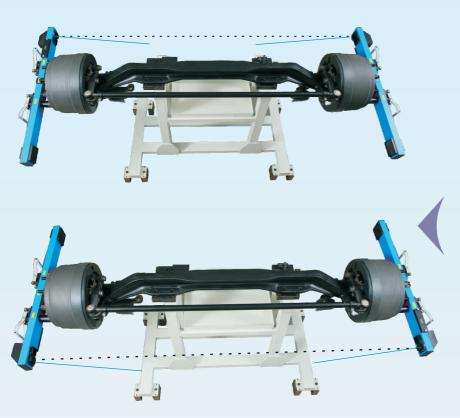
The camera hub adaptors should be mounted on respective sides (LH & RH) of the axle & the software will guide the user to acheive the horizontability of the Camera hub adaptors, to set the straight ahead position first and then rotate the hub adaptors by 180 degree to compensate the static errors. The measurements will be taken in both front & rear side of the axles. The system will measure individual toe of each axle hub independent of the distance between the axle hubs.
