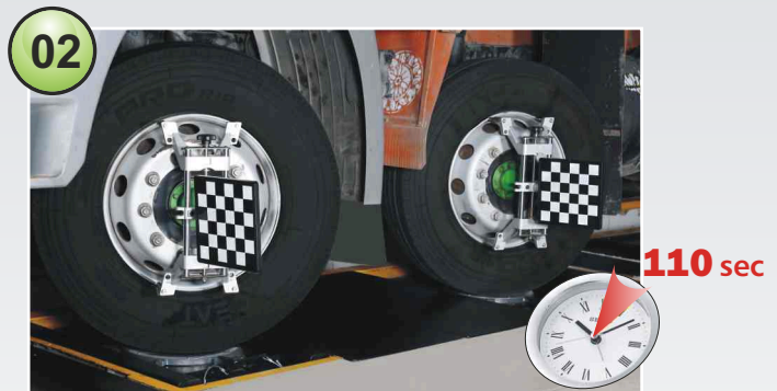
One shot Caster swing of twin steer axles
